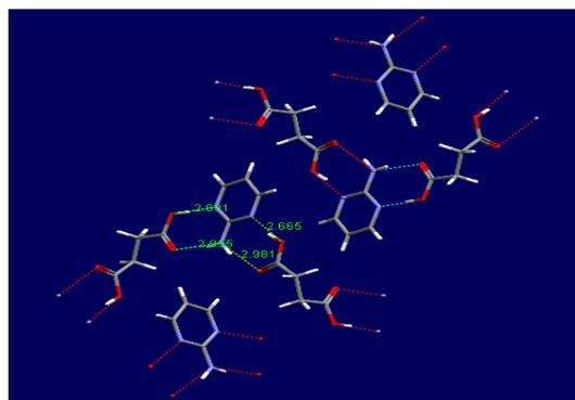
**Figure 2.** A packing diagram for 2-aminopyrimidine succinic acid, viewed along the *a* axis<sup>[6]</sup>.
