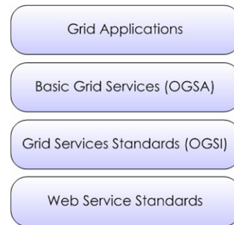
Figure 1: Grid application stack
