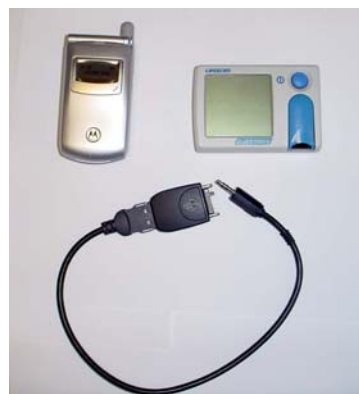
Figure 3: Diabetes self-management system: mobile phone, blood glucose meter and cable
